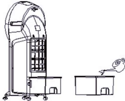
3. Replace the tank back onto the back of the unit. Turn the water tank knob clockwise 90°. This locks the water tank back into place.
