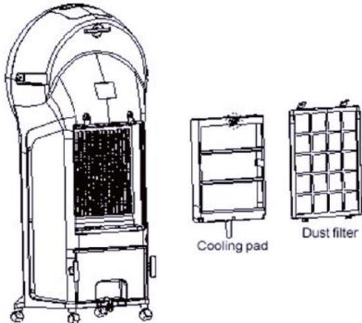
1. Remove the dust filter from the back of the unit by pushing down on the two tabs located above the filter and pulling it out. Gently scrub it with a soft brush and rinse with water.
